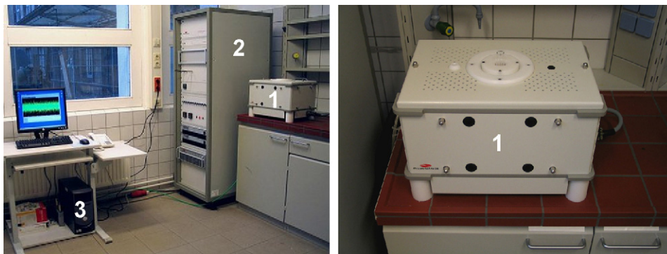
Fig. 1. (Left) NMR-MRI-Benchtop system consisting of the (1) temperature controlled permanent magnet with resonator, (2) power supply and electronic accessories and (3) computer and (Right) permanent magnet with resonator.
